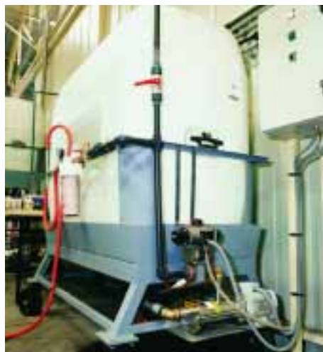
Compact M2200C4 for feeding salted water installation.
