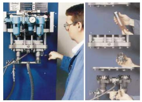
The plungers and packing glands can be easily replaced on-line in 20 minutes.
