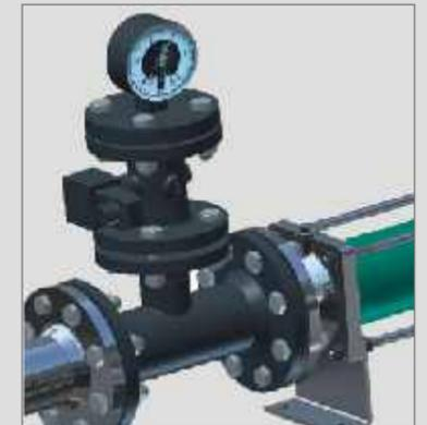
Display of operating pressure by a bourdon gauge. Gauge is isolated from the process fluid by an elastomer diaphragm. Shut down of the pump when the maximum allowable pressure is exceeded with adjustable pressure setting. Also available with a differential pressure on/off switch.
