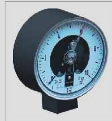
The pressure gauge displays the operating pressure. Gauge is isolated from the process fluid by a stainless steel diaphragm. Shut down of the pump when the maximum allowable pressure is exceeded with adjustable pressure setting. Suitable for low up to medium viscosities.
