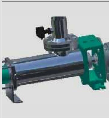
The flow sensing unit is used to protect a progressing cavity pump fitted with a solid stator against dry running. The unit senses the flow in the suction or discharge pipework. Should the flow drop below a predetermined level, indicating a dry running situation the unit will shut down the pump, thus preventing any damage.
