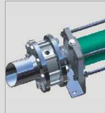
For the transportation of high viscosity media we recommend the installation of our ring dosing nozzle. The nozzle fits directly to the discharge connection of the pump and allows the injection of a boundary layer lubricant. Depending on the lubricant used the pressure loss in the discharge pipework can be reduced by up to 70% in comparison to operating the system without any lubricant injection. By operating this system both the investment and operating costs are significantly reduced.
