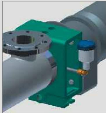
A quench pot is necessary when a shaft seal needs to be operated with a quench, but it is not required that the seal has a permanent flushing flow. So that dry running of the seal or crystallisation of the pumped product can be prevented we recommend the installation of a quench pot.
