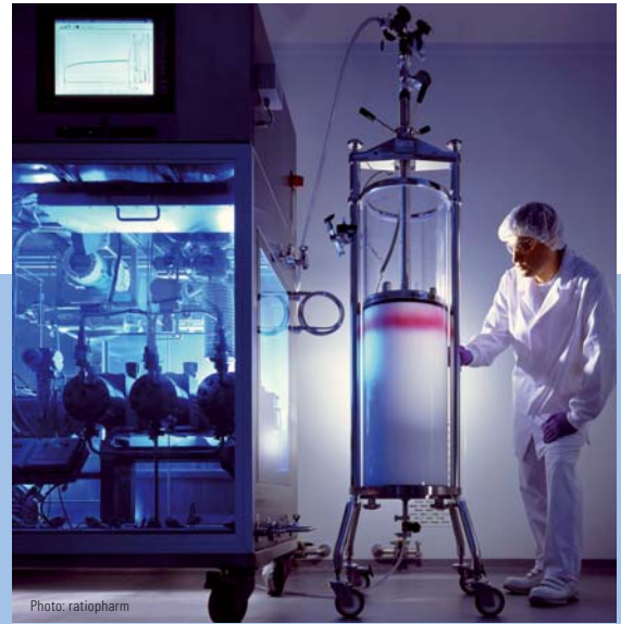
By intelligently overlaying the feed flows of two single pumps, it is possible to prevent pressure pulsation, even without pulsation dampers.
