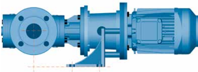
Conversion situation 1: The electric motor is unchanged: the same output and size. The KRAL flange to take the VDMA connecting frame makes the unit a bit longer. The pump pedestal is the same as it was for the pump with a mechanical seal. The pipe connection dimension is the same. The change in length is compensated by adapter sleeves, so that the pedestal mounting dimension is retained.
