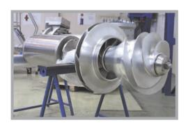
The pump rotates in the counter clockwise direction viewed from the pump inlet and is driven by the electric motor, a form wound, squirrel cage, 6,600 V, 4 pole, driver designed to operate in cryogenic fluid.
