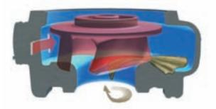
Stage two: rags get fed into the relief groove as the impeller turns, pulling them from the impeller and forcing them into the volute where they get pumped away.
