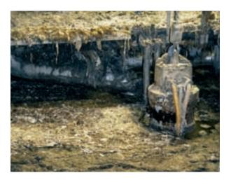
Flygt submersibles operate directly in the pumped liquid. This means low construction costs because Flygt pumps don't require a special housing or a superstructure. Operating submerged also means that our pumps take up very little space, are quiet and do not need extra cooling.
