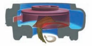
The two-stage action is designed to prevent rags and other fibrous material from accumulating on the impeller.
