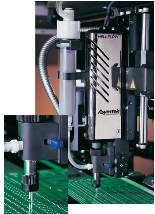
The DV-7000 Heli-Flow® pump is available in a luer- or footed-needle design with interchangeable cartridges, allowing each pump to work with several different fluid types. The DV-7000 has a hardened auger for use with filled epoxy materials and features a high flow rate.
