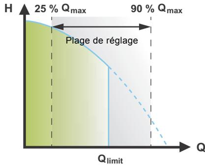
Fig. 27 FLOW<sub>LIMIT</sub>
