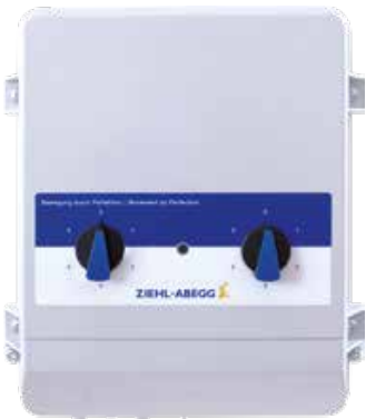
Transformer based controllers 1~ with two 5-step-switch, two speeds external changing 1~ 230V 50/60Hz
