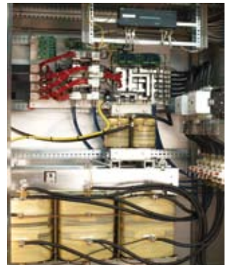
Power supply unit including medium frequency converter and high voltage transformer
