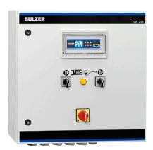
The CP 221 is a control panel providing a complete solution for 2-pump sewage pumping stations. It is built around the PC 242 controller with advanced control and monitoring features to give optimum performance and reliability over the stations whole life cycle. It is designed to be wall mounted in buildings and the design will give a high degree of redundancy to maintain pump operation in most cases of single failure.
