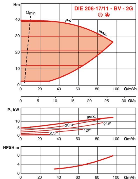
**PERFORMANCES HYDRAULIQUES - FONCTIONNEMENT EN MODE NORMAL / SECOURS**
