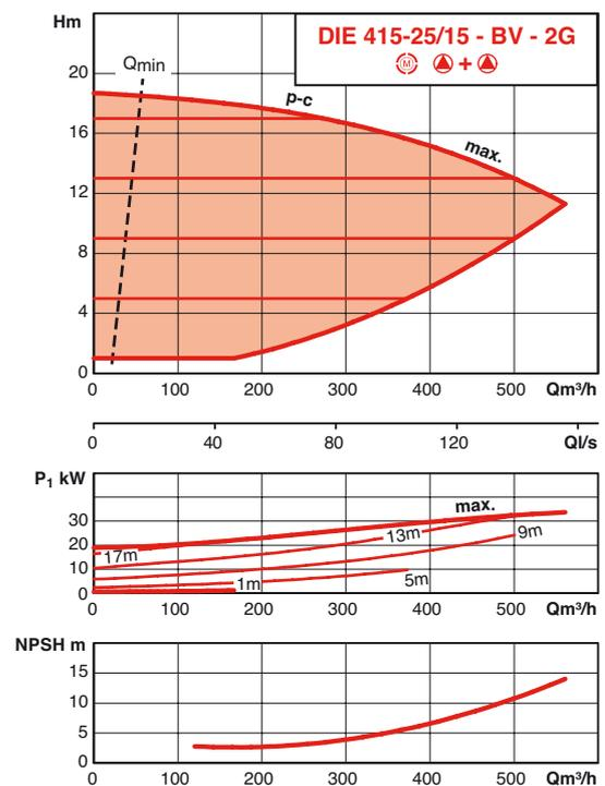
**PERFORMANCES HYDRAULIQUES - FONCTIONNEMENT 2 POMPES EN PARALLELE**
