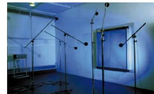
Noise measurements to DIN 45 635-38 „Noise Measurement of Machines: Fans“
