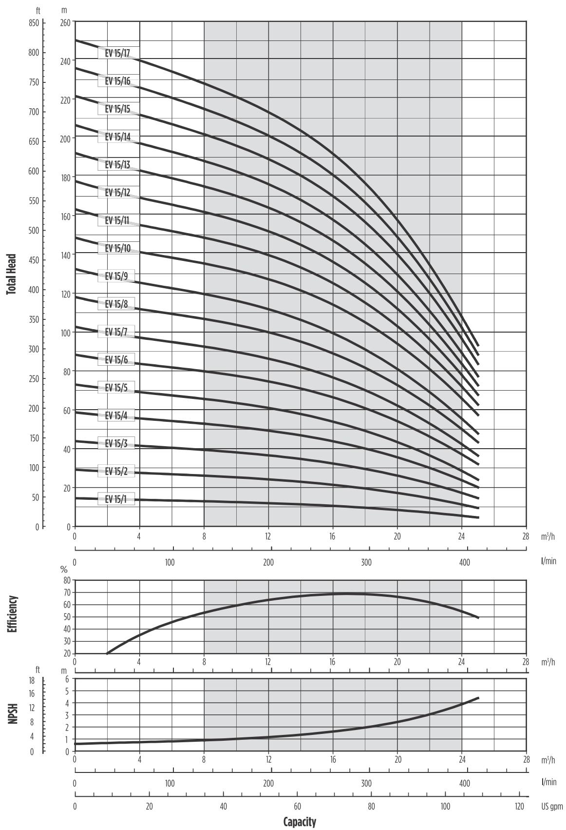
The hydraulic characteristics are guaranteed, according to ISO standard 9906:2012, grade 3B
