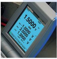
Selected modes and functions, as well as physical and electrical values, and relevant warning symbols, are all clearly displayed on the instrument's 160 x 160 highresolution graphic display.
