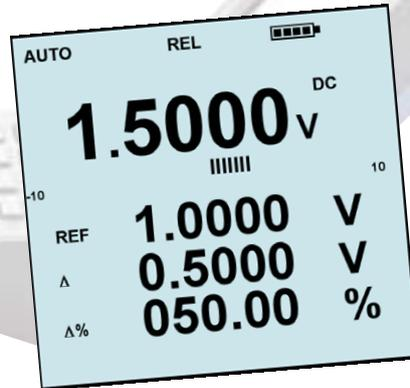
Thanks to the instrument's 4 digital displays, the relative function **REL** provides comprehensive simultaneous display of the absolute and absolute drift values, relative drift % and reference value.
