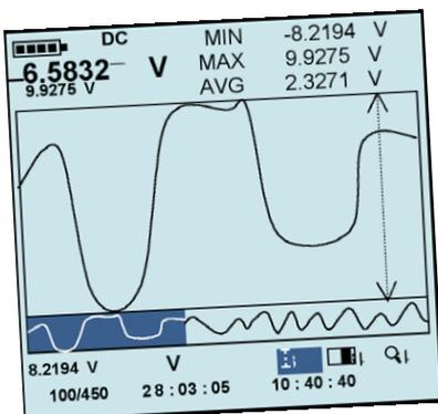
The **MEM** function enables you to record up to 6500 date/time measurements, for periods ranging from 1 sec to 24 hrs, and to analyse the results graphically for up to 4 simultaneous measurements.
