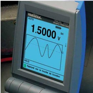
A "preferred measurement" key
