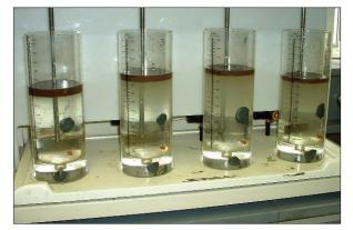
The Leopold Jar Testing Unit is a stand-alone system designed to test four samples independently and simultaneously, giving flexibility and variable control.
