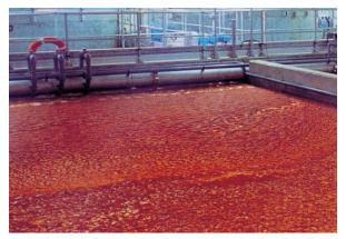
The next step for this sludge produced by a Clari-DAF LT system is dewatering where higher cake solids result in lower disposal cost.
