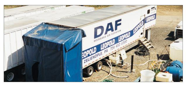
The Leopold mobile Clari-DAF system pilot plant gathers data every five minutes around the clock for weeks under actual operating conditions to determine the most appropriate flocculation conditions for designing and engineering a full-scale Clari-DAF system installation.
