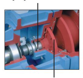
EXPELLER - the Equiseal® dynamic seal uses an auxiliary expeller in the seal chamber. As pumped liquid enters the dynamic seal stuffing box cavity, it is opposed by centrifugal force, generated by the auxiliary expeller creating a liquid sealing ring, thus preventing leakage.
