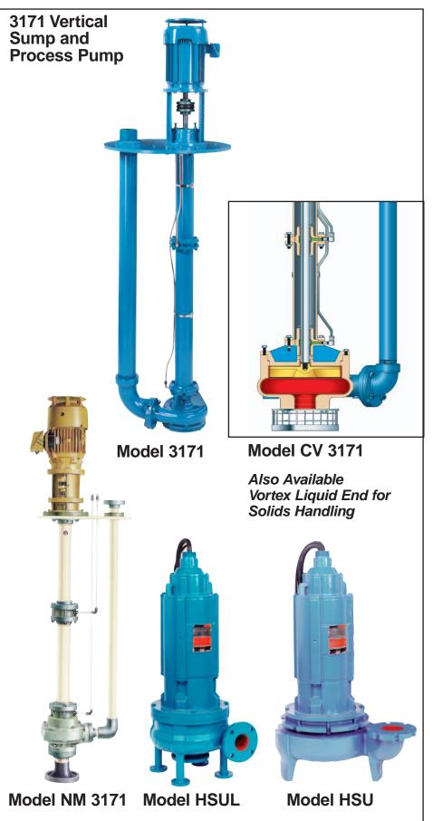
Goulds Pumps offers a wide range of sump pumps in submersible and wet pit designs. The 3171 line offers metallic constructions from cast iron to CD4MCu and non-metallic FRP. Also offered is a recessed impeller design specifically for solids handling.
