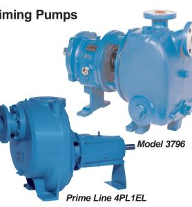
The Self-Priming pumps are available in sizes from 2" to 12" (76 mm to 300 mm) with capacities to 6,000 GPM (1,375 m³hr) and heads to 200 ft (60 m). The solids handling, non-clog impeller is capable of passing solids up to 3" (76 mm). Designed to provide maximum uptime and ease of maintenance, these rugged pumps are constructed of cast-iron, 316 stainless steel or hard metal CD4MCu. Trash Hog is perfect for pumping raw sewage, sludge and wastewater.
