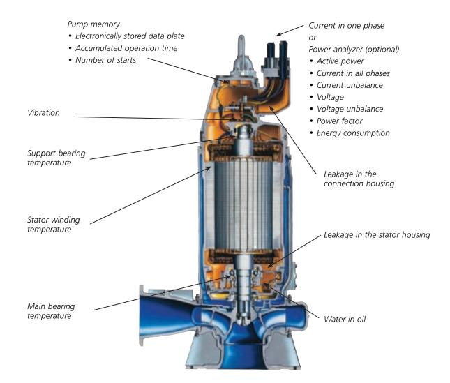
Flygt MAS 711 monitors and stores measurements from the customer's selection of factory-installed sensors. In addition, essential data about the pump useful for installation, servicing and maintenance (stored in the pump memory) is automatically synchronized with the corresponding data in the base unit every two hours. Flygt MAS 711 uses the pump's data plate information stored electronically in the base unit and the pump memory to authenticate the pump during synchronization.
