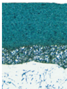
Cross section of Flygt epoxy coating
