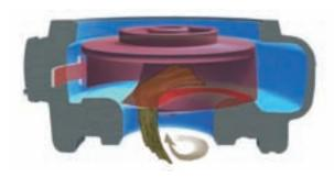
The two-stage action is designed to prevent rags and other fibrous material from accumulating on the impeller.
