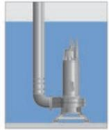
**NS** – This installation makes the pump easy to move around with either a flange that connects to a discharge pipe or a hose coupling.
