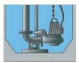
It hasn't changed for over 30 years: a large flat sump floor that encourages the build up of sludge and
