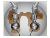
Solids that are left behind will collect close to the pump, where the suction is the strongest. This means they will not have the chance to build up and stagnate.
