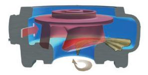
Stage two: rags get fed into the relief groove as the impeller turns, pulling them from the impeller and forcing them into the volute where they get pumped away.
