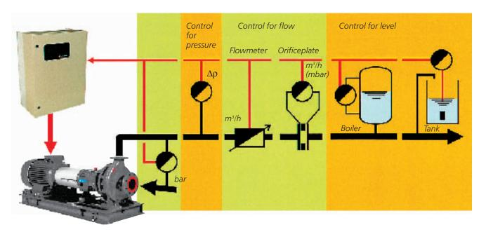
At controller mode "normal" the operating frequency will be increased in case the measurement signal decreases.
