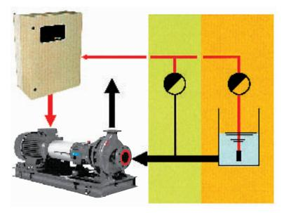
At controller mode "inverse" the operating frequency will be decreased in case the measurement signal decreases.
