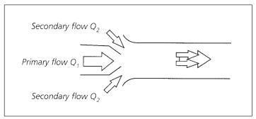
2. When the liquid level is lowered and the jet breaks the surface, the Flygt Jet Mixer becomes a flushing device. The flow (Q1) passes through the nozzle and the ejector pipe, resulting in a powerful jet which cleans the basin floor and walls.
