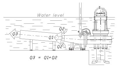
When the water has dropped to the level at which the pipe is no longer totally submerged, the flow from the pump helps flush the basin floor.
