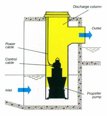
Pump and motor are a complete unit
