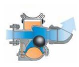
During the next 20 seconds, the ball is lifted by the membrane as the pressure in the two chambers equalizes. The time this takes can be varied by regulating the oil flow from the oil reservoir to the chamber beneath the membrane.
