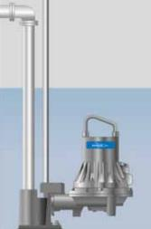
Stationary wet installation with guide bars and automatic discharge connection bolted to the sump floor. When lowering a pump with guide bars, the pump automatically locks to, and is released from, the discharge connection.
