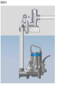
Stationary wet installation with the pump suspended from the discharge pipe. The quick connection joint has an integrated non-return valve.
