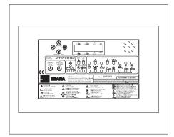
Digital remote control unit control panels for monitoring the alarms in the manned place to be connected to the FFP control panels and the solenoid valves of the fire-fighting unit.
