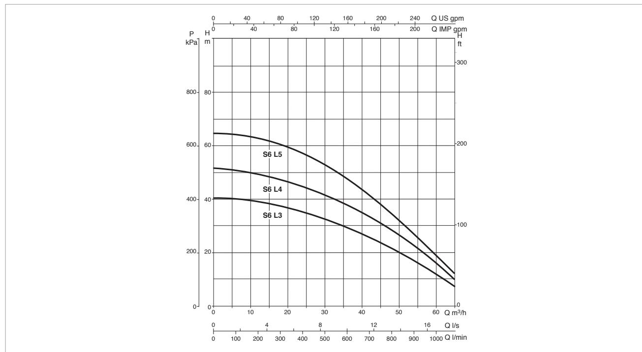
The performance curves are based on kinematic viscosity values = 1 mm<sup>2</sup>/s and density equal to 1000 kg/m<sup>3</sup>. Curve tolerance according to ISO 9906.
