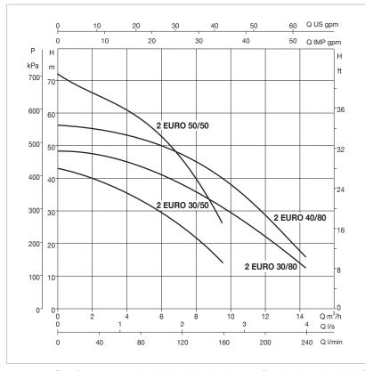
The performance curves are based on kinematic viscosity values  $= 1 \text{ mm}^2/\text{s}$  and density equal to  $1000 \text{ kg/m}^3$ . Curve tolerance according to ISO 9906. **Overall performance taking into account TWO pumps working at the same time.** The performance results of sets with smaller pumps (e.g. 2 EURO 40/50) are obtained through simple calibration of the AD module.
