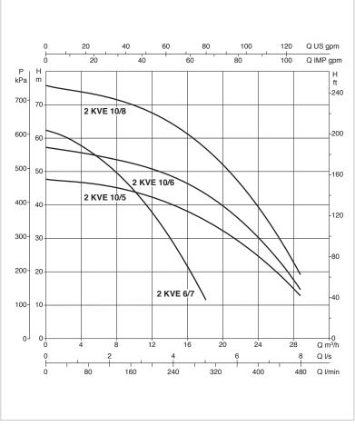
The performance curves are based on kinematic viscosity values = 1 mm2/s and density equal to 1000 kg/m3.
