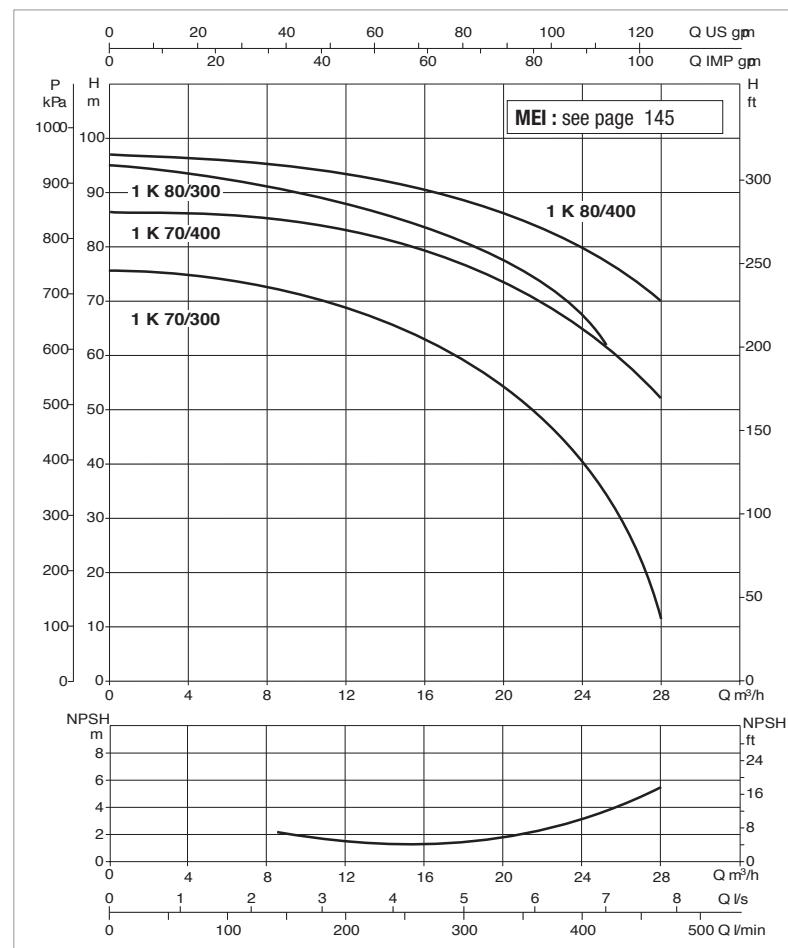
The performance curves are based on kinematic viscosity values = 1 mm<sup>2</sup>/s and density equivalent to 1000 kg/m<sup>3</sup>. Curve tolerance according to ISO 9906.
