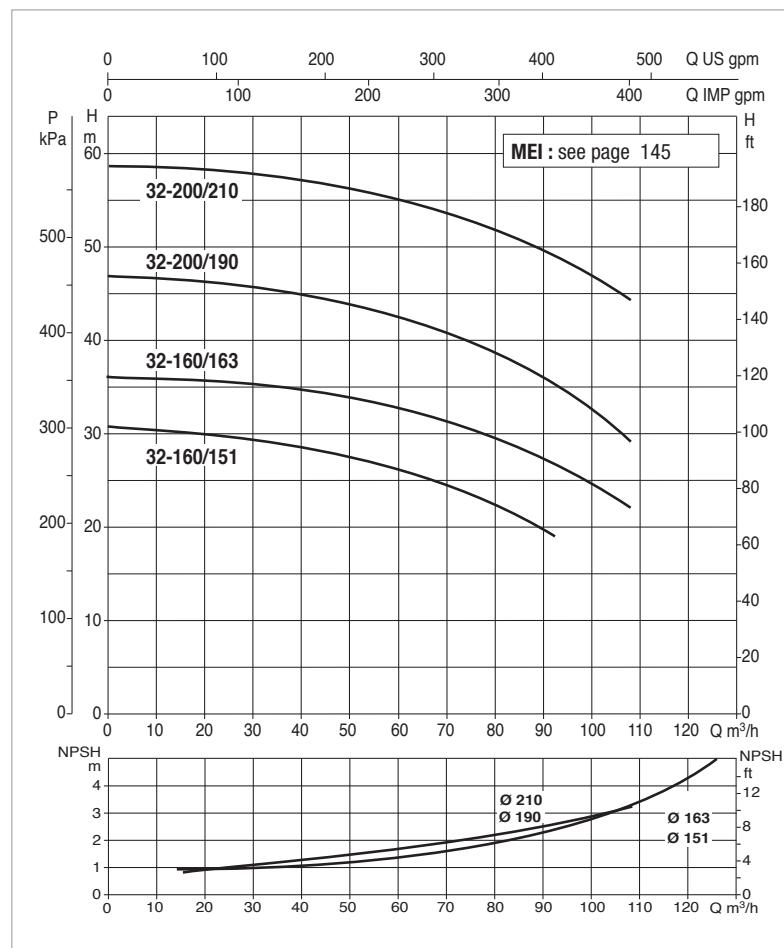
The performance curves are based on kinematic viscosity values = 1 mm<sup>2</sup>/s and density equivalent to 1000 kg/m<sup>3</sup>
