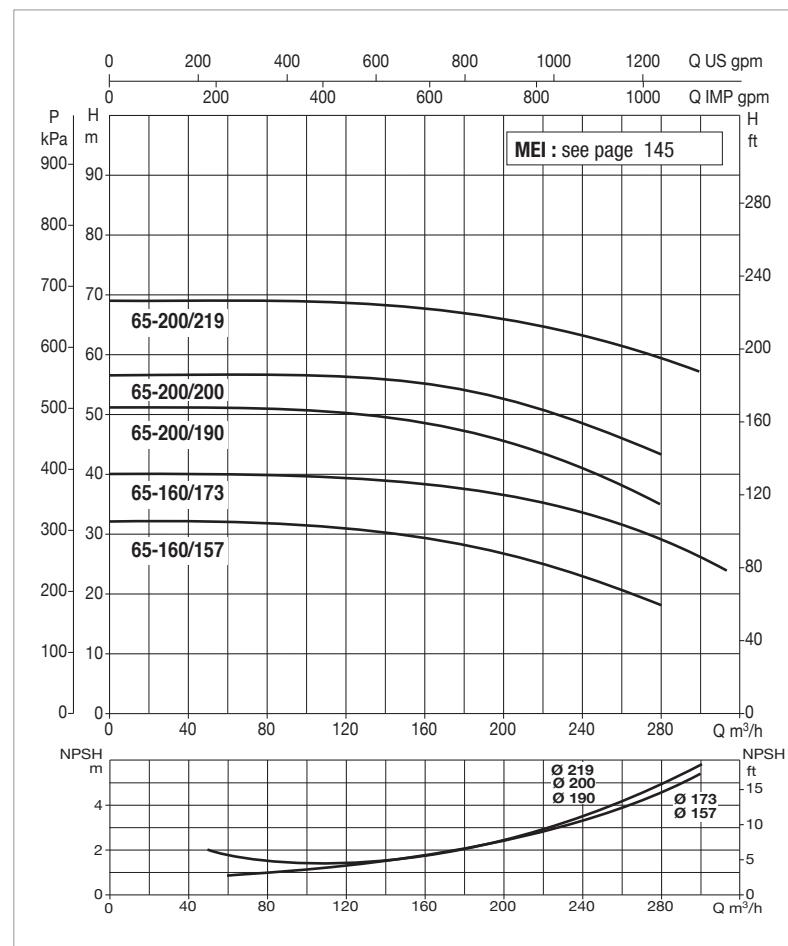
The performance curves are based on kinematic viscosity values = 1 mm²/s and density equivalent to 1000 kg/m³
