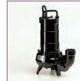
Electric pumps with set back opening impeller or vortex type and with generous free passages are ideal for handling screened water, effluent or for emptying small community septic tanks. Vortex type impeller versions are recommended where the liquid pumped contains solid matter in suspension or fibre.
