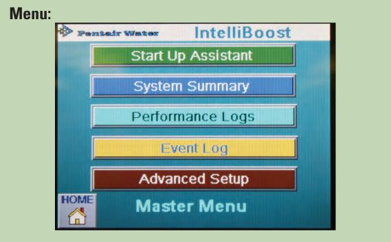
Fast and Easy Start-up with the 3.8" inch touch screen control HMI (humam machine interface) panel operation.
