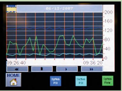
The performance log consists of a graph of flow, suction pressure, and discharge pressure, plotted against time, with continuous update in real time. Data is retained for future review. The screen shown is the 5.7" color screen and is in enhance mode.
