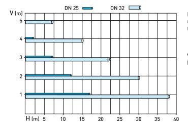
Maximum pipe length allowable for the optimum functioning of the unit. Allowance has been made for two  $90^\circ$  bends and one Sulzer non-return valve.
