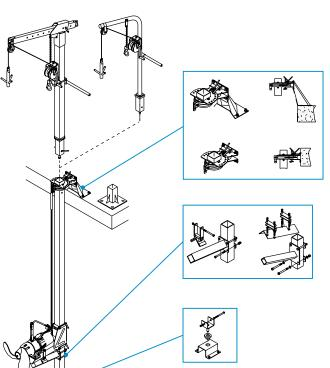
The mixer is supplied as standard with a runner and hoisting hook. All structural work can be supplied in hot-galvanized iron or stainless steel.
