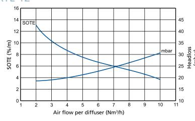
EPDM LP membrane. fine bubbles Oxygen transfer according with ATV M209 Density 5.3%
