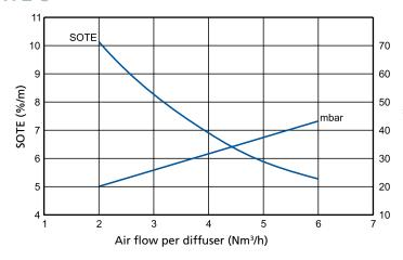
EPDM LP membrane. fine bubbles Oxygen transfer according with ATV M209 Density 6.5%
