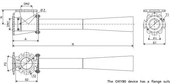
The OXY80 device has a flange suitable for connection to electric pumps having delivery DN80 and DN100.
