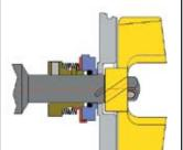
Type D External Balanced Seal This versatile, dependable seal finds broad use in sanitary and industrial applica-
