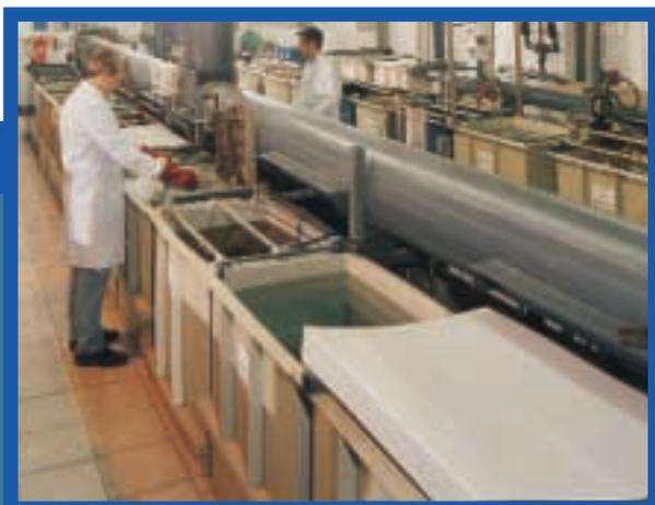
A leading alloy wheel manufacturer, identified a problem in its pre-treatment plant which was the cause of unacceptably high rejected product. More **accurate and reliable** metering of various aggressive chemicals such as deoxidants, hydrofluoric acid, detergents and chromate solutions was required.
