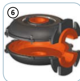
Pump body Impeller and pump body in GJL-250 cast iron coated with abrasion-resistant polyurethane (Vulkollan)
