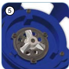
Cutter Grinder system comprising a revolving cutter and a plate with holes with sharpened edges that fine-chops filaments, preventing fouling of the impeller
