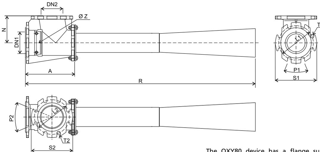
The OXY80 device has a flange suitable for connection to electric pumps having delivery DN80 and DN100.
