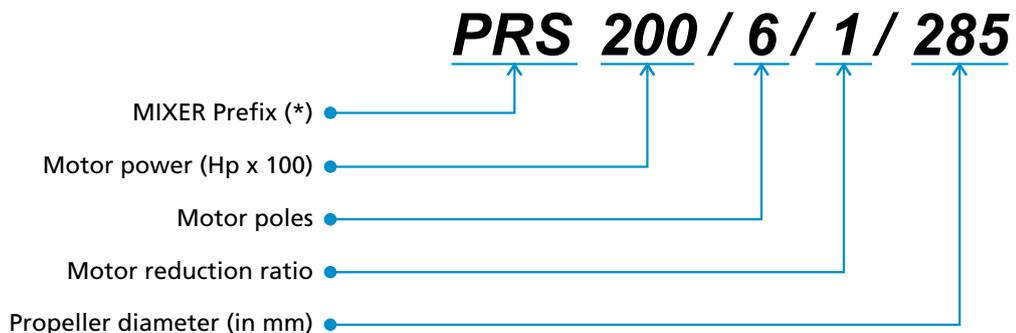
(\*) PRS - cast iron casing - direct transmission
