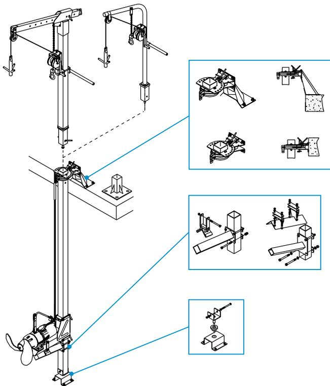
The mixer is supplied as standard with a runner and hoisting hook. All structural work can be supplied in hot-galvanized iron or stainless steel.
