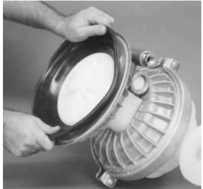
Step 10. Figure 10 Using an adjustable wrench, or by rotating the diaphragm by hand, remove the diaphragm assembly. ( Figure 10 )
