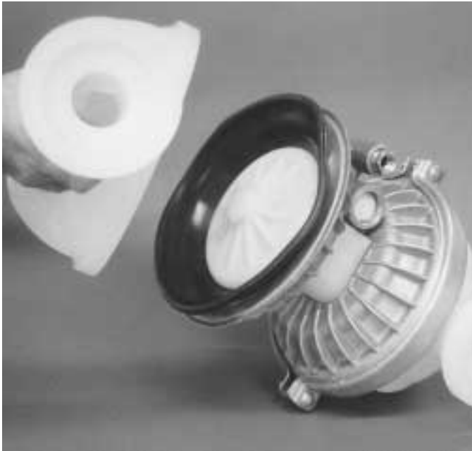
Step 9. Figure 9 Lift liquid chamber away from center section expose diaphragm and outer piston. ( Figure 9 )
