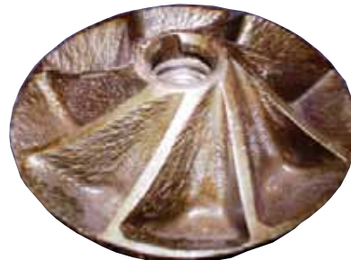
Cup-type impeller - after thousands of hours of service, vane and cup areas increase.
