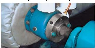
For low pressure transfer of clean blended or cutback asphalts, Viking offers jacketed General Purpose asphalt pumps. The "floating" rotor on these pumps is a simple, economical design.
