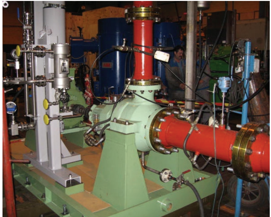
MPP-OHH pump being performance tested with a multiphase mixture of water and nitrogen
