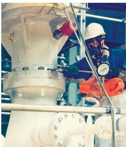
Liquid nitrogen cold spin test
