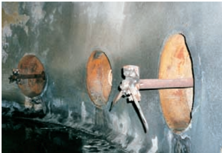
Fig. 2. Agitator with too short a shaft has lost one propeller blade. The farthest agitator has lost all three blades and the one in the middle is in the workshop. All these agitators had 30 kW motors and 1000 mm propellers. All of them suffered from frequent fatigue failures.
