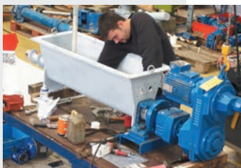
Revamping of a Moineau pump GBB series with installation of the new bridge-breaker device
